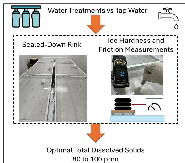
These investigations take place on a purpose-built, scaled-down experimental rink that allows environmental and operational variables to be carefully controlled. By producing ice across a defined range of total dissolved solids and evaluating it using non-destructive measurements, the work provides
