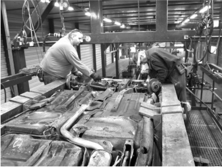
Figure 3 Station 4 of the system (see Figure 1) where cars are turned upside down for engine and gearbox unfastening.
