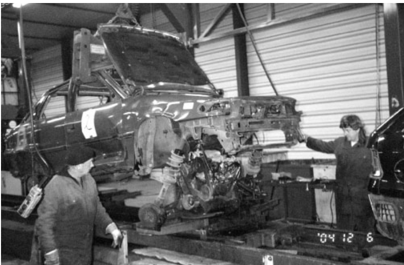
Figure 4 Station 5 of the system where the engine and gearbox are removed following release at station 4 (see Figure 3).
