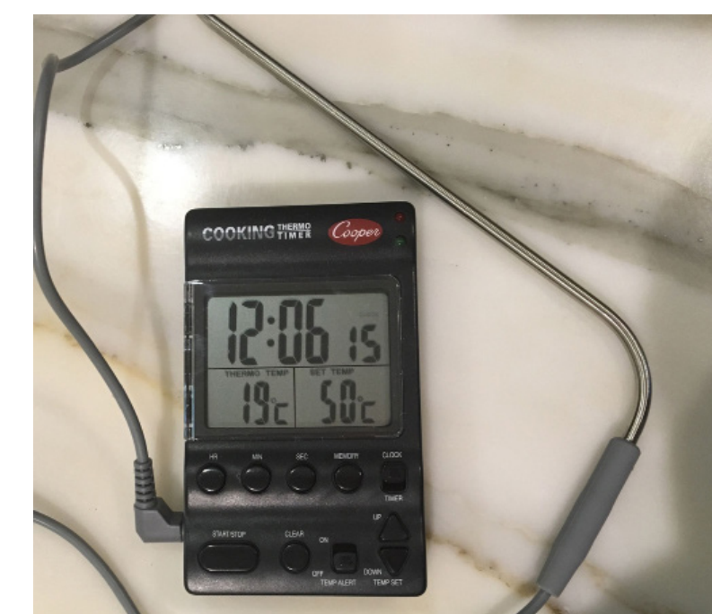
Figure 1. Digital probe thermometer used for recording milk temperatures
