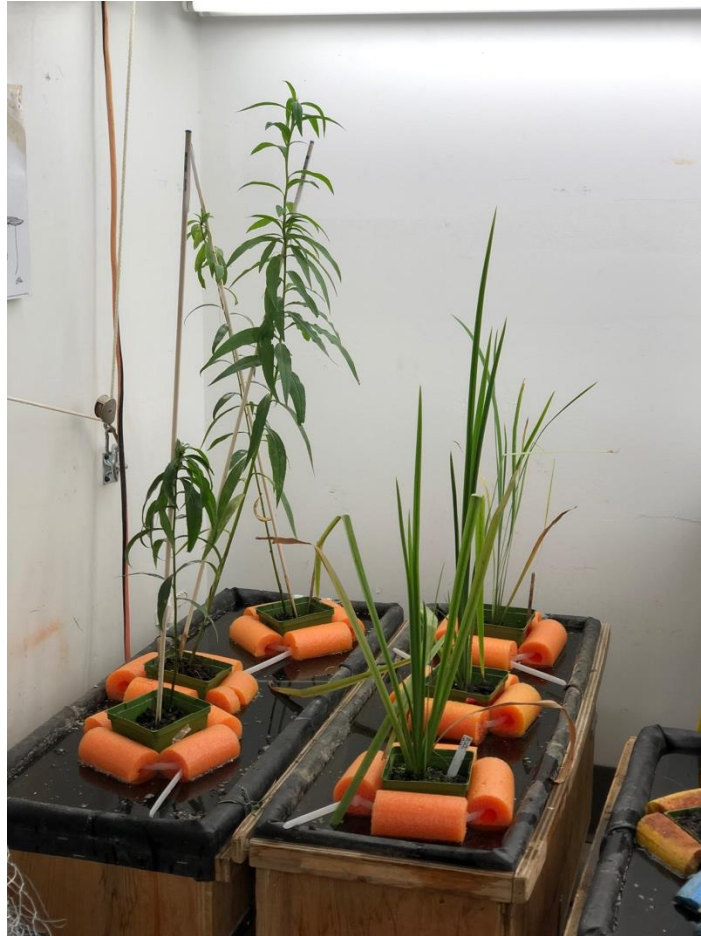
Figure 7: Experimental Setup of Floating Engineered Wetland System
