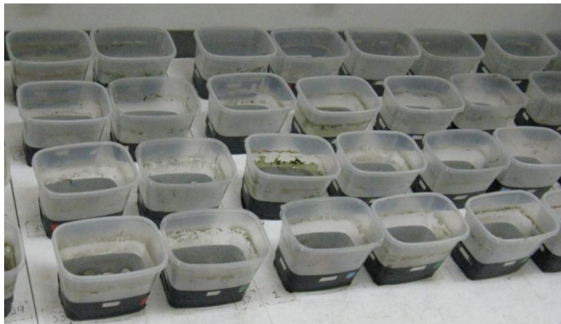
Figure 16. Microcosm vessels with black duct tape covering the lower 6 cm of each vessel and identifying labels after the removal of Typha latifolia shoots.
