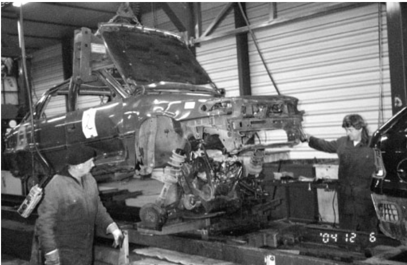
Figure 4 Station 5 of the system where the engine and gearbox are removed following release at station 4 (see Figure 3).
