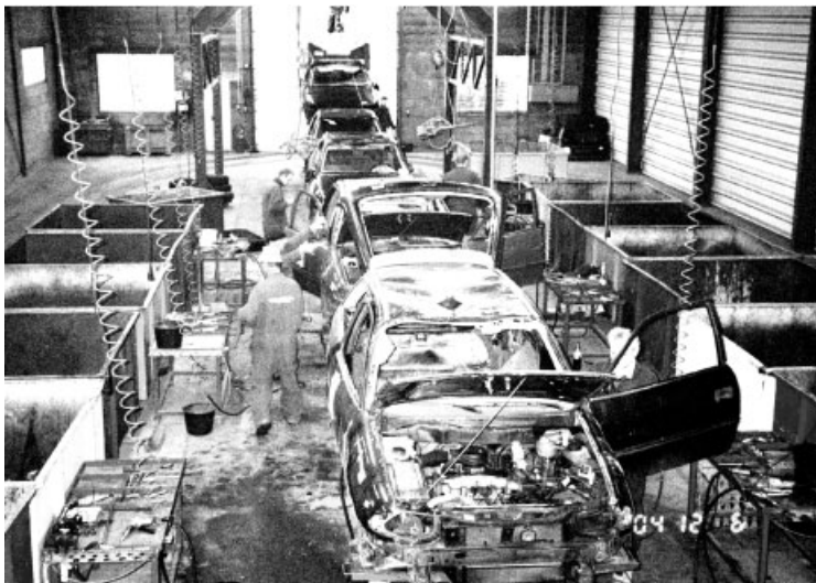
Figure 2 Stations 1–3 of the system where glass, rubber, and interior materials are removed. Containers for disassembled components and material are on each side of the line.
