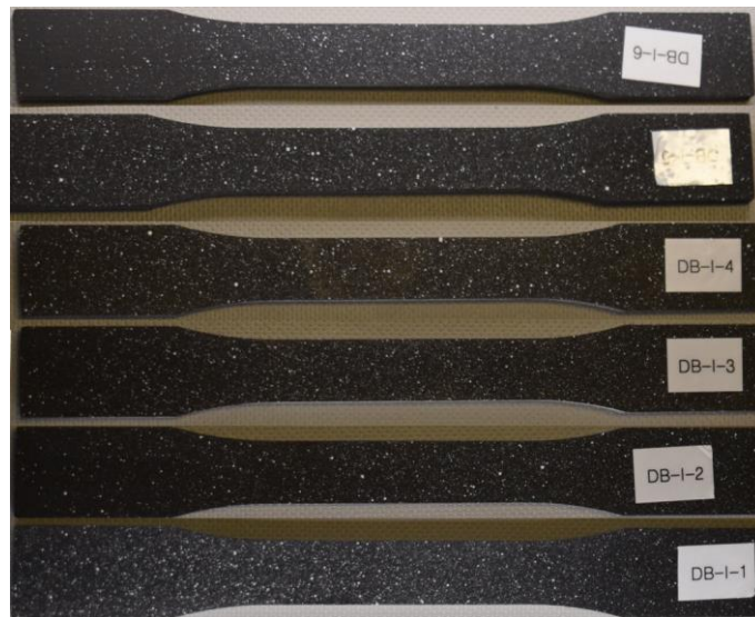
Figure 6. ABS Type I dog-bone tensile testing samples after painting black and speckling on one surface.
