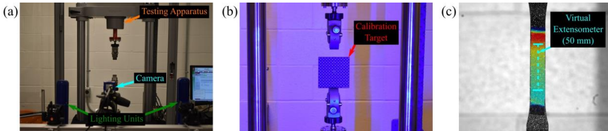
Figure 7. DIC imaging procedure: (a) Imaging setup for tensile testing; (b) Calibration setup; and (c) Representative DIC strain field.
