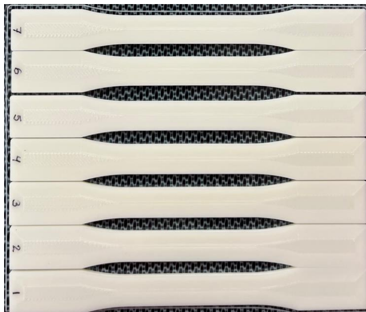
Figure 5. 3D-printed ASTM D638 Type I specimens after the MEX additive manufacturing.
