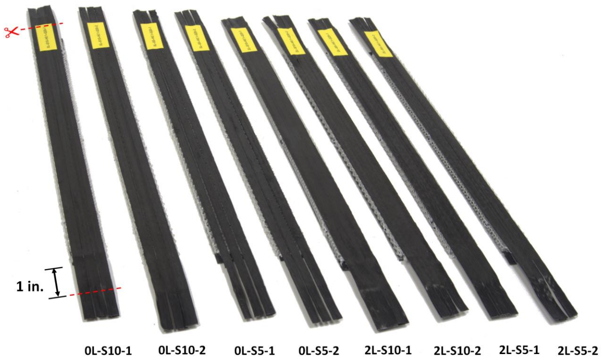
Figure 4. In-situ consolidated sandwich specimens for climbing drum peel with extended skins.
