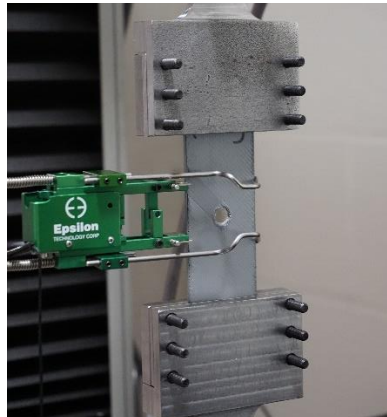
Figure 9. The test set-up including a variable stiffness specimen ( w/D=4 ), the fixture, and the extensometer.
