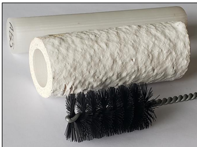
Fig. 2. Materials for friability measurement: 3D-printed ABS pattern, ceramic shell after burnout (700 °C), and test brush.
