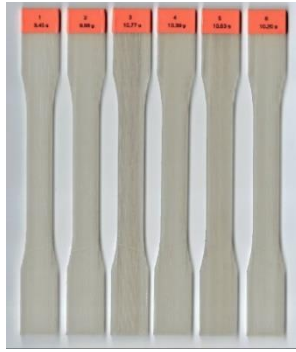
Fig. 3. Six 3D printed specimens out of extruded filaments.
