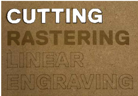
This sample shows the three different techniques on the same material.
