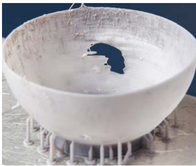
Example of blowout due to "suction cupping."
