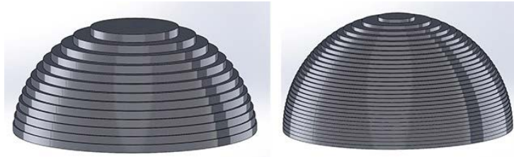
Visualization of layer thickness comparison.
