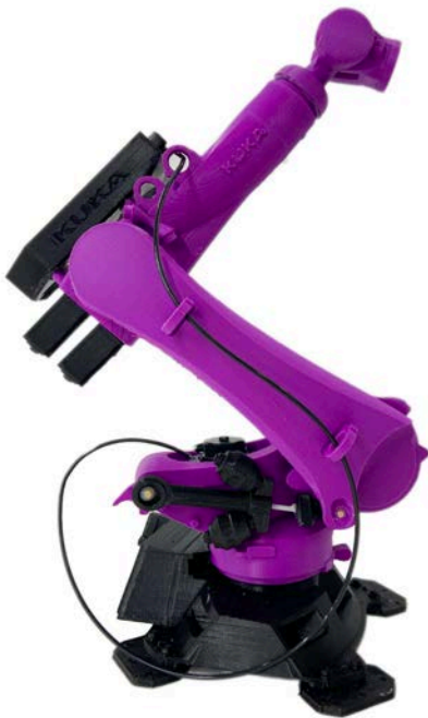
A 3D Printed Articulated Kuka Robot arm.
