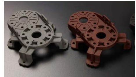
SLS print vs. SLS print dyed with Rit Dye.
