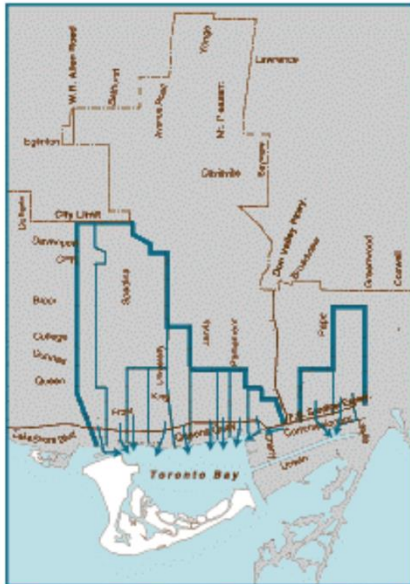
Figure 2: Combined sewer map. All outflows are highlighted in blue. As you can see on this map, there are numerous outflows located in the Toronto Harbour basin that are close to the north side of Toronto Island.
